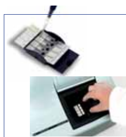
3. Pipette to test chips and start the GenomEra CDX™ assay run
