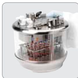
Combined reflux and additions head with nickel condensing fingers
